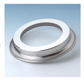
LJ Star's ASME Section VIII rated Sanitary Clamp adheres to the highest engineering standards, to ensure uniform clamping compression for an observation window installed in a high-pressure system. The clamp is cast from 316 stainless steel. It features a heavy-duty three-bolt and hinge design for safe operating systems, while allowing quick access to joints for cleaning and/or inspection.
