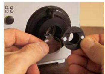
Bezel accepts filters too! Install IR and/or long term use filters here.
