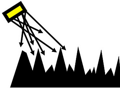
Figure 10: Soft light hitting a rough surface at a variety of angles. None of the surface experiences shadowing or masking.
