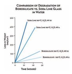
Standard DIN 7080 rates borosilicate glass to 280 C (536 F) and Standard DIN 8902 rates soda lime sightglass to 150 C (302 F). Very high-temperature equipment, such as ovens and furnaces, may require windows made of quartz. The following chart compares the maximum operating temperatures of glass commonly used in sight windows.
