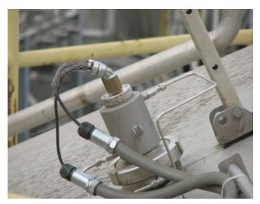
Figure 3. Camera installed in an air-cooled housing.
