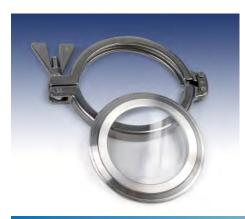
A sight window made from an optical grade polymer formed into a stainless steel ring. It mounts via a sanitary clamp that speeds removal during cleaning. MetaPlex® sanitary windows offer greater toughness and temperature performance. Ideal for food & beverage, brewery, chemical and pharmaceutical applications.
