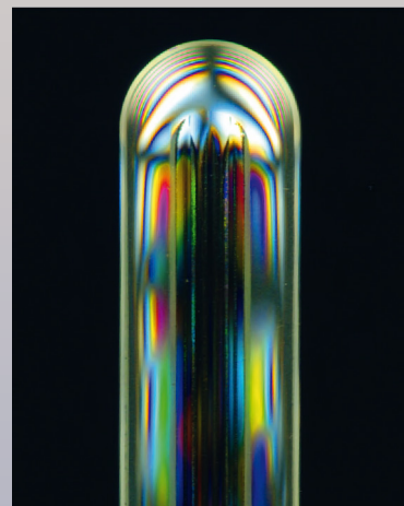
Special tempered MAXOS® glass under polarized light.
