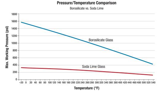
This chart shows the operating temperature of a fused Borosilicate sight glass and fused Soda Lime sight glass at different temperatures. (From "Compression vs. Fusion in Sight Glass Construction" by Karl Schuller, Herberts Industrieglas GmbH. Used by permission.)
