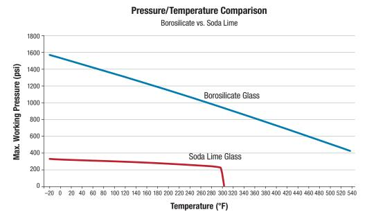
This chart shows the operating temperature of a fused Borosilicate sight glass and fused Soda Lime sight glass at different temperatures. (From "Compression vs. Fusion in Sight Glass Construction" by Karl Schuller, Herberts Industrieglas GmbH. Used by permission.)
