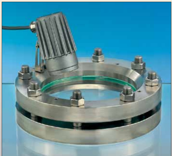
Combination light/sight glass assembly on circular sight glass fitting type DIN 28120; luminaire mounted with hinged bracket
