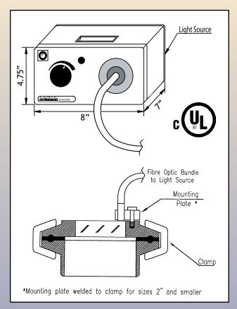
powerful yet compact illumination system for sanitary processing equipment provides up to 150 Watts of adjustable illumination while allowing viewing through the same window. These unique combination units incorporate the L.J. Star MetaClamp<sup>®</sup> system with Metaglas<sup>®</sup> safety windows. They can be used to view the interior of either new or existing sanitary processing equipment.
