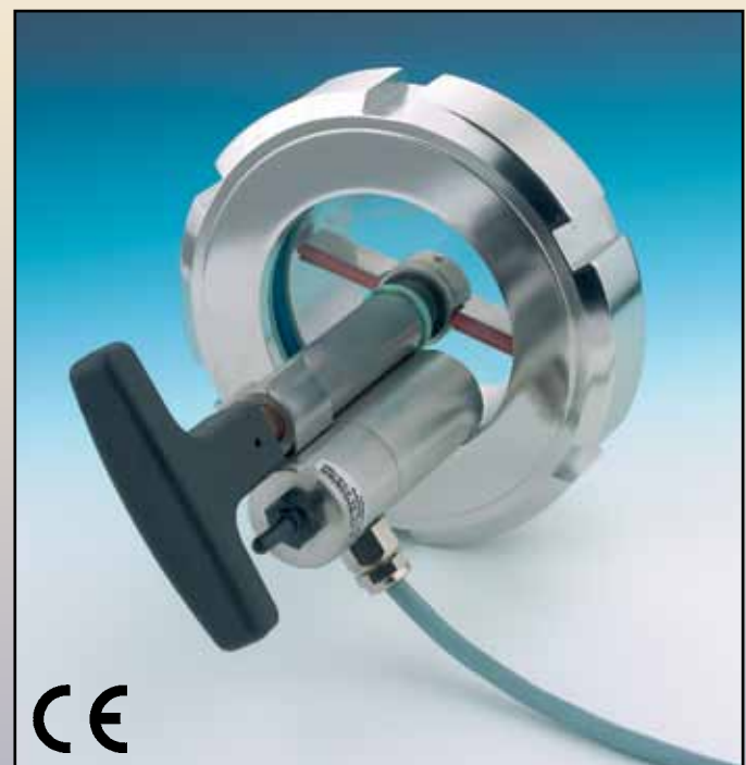
Lumiglas Stainless Steel Mini-Luminaire, Series USL 01 with mounting clamp fitted on a screwed sightglass fitting with Lumiglas sight-glass wiper type SW I.
