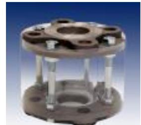
**View-through flow indicator.** This type of flow indicator has two opposing windows so that an operator can see the intervening flow of fluid lighted from behind, either by ambient light or with an attached luminaire. Unlike 360-degree full-view flow indicators, this design is suited for ANSI pressure classes, high temperature, and harsh fluid applications.
