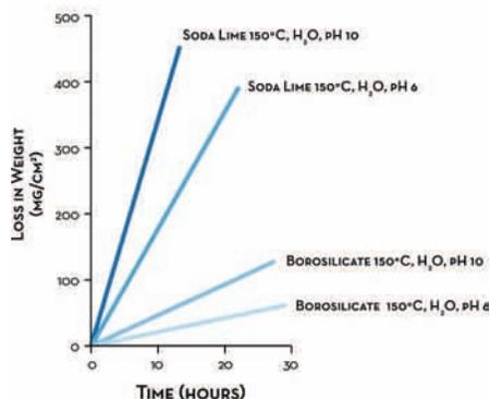
Standard DIN 7080 rates borosilicate glass to 280 C (536 F) and Standard DIN 8902 rates soda lime sightglass to 150 C (302 F). Very high-temperature equipment, such as ovens and furnaces, may require windows made of quartz. The following chart compares the maximum operating temperatures of glass commonly used in sight windows.
