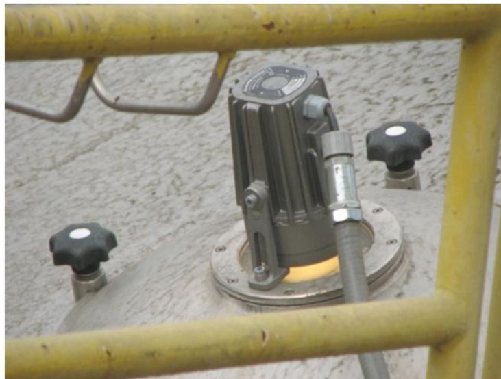
Figure 2. High intensity discharge lamp lights the inside of the whirlpool tank.
