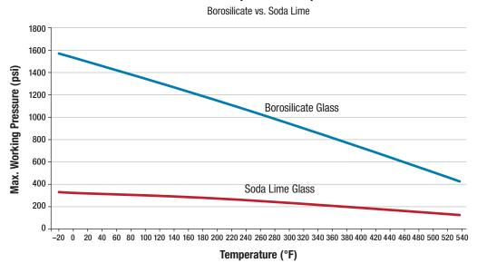
This chart shows the operating temperature of a fused Borosilicate sight glass and fused Soda Lime sight glass at different temperatures. (From "Compression vs. Fusion in Sight Glass Construction" by Karl Schuller, Herberts Industrieglas GmbH. Used by permission.)
