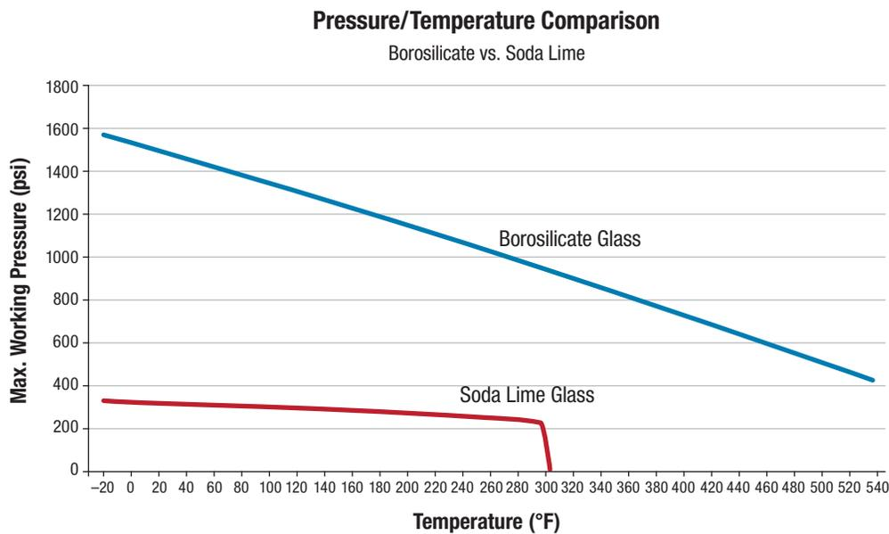
This chart compares a sight glass comprised of duplex stainless steel and borosilicate glass with a sight glass comprised of Hastelloy C-22 steel and soda lime glass. The sight glass that uses borosilicate glass is many times stronger across a range of operating temperatures.
